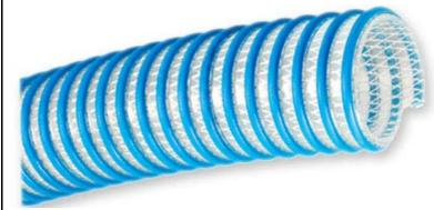
The Model UH1 Hose is a made from thick polyurethane to provide one of the most durable material handling hoses. Blue PVC external helix and embedded wire. FDA food grade materials. 3" to 6" diameters
